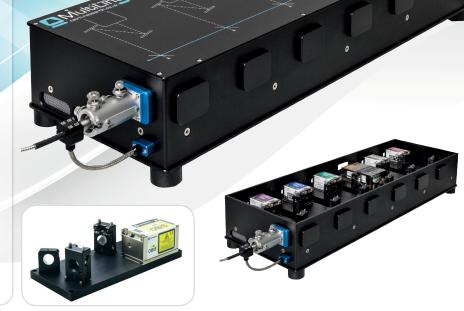
The system can accommodate up to six lasers which can be combined into up to eight different fibres with arbitrary light distribution or sharing of wavelengths between ports. Mechanical shutters and galvanometer switching modules are available as required. The lasers can be controlled using the Cairn MultiLine controller with computer and / or front panel digital and analogue modulation, or used with the laser manufacturer or other third-party power supply.
