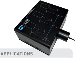
The system can accommodate up to six lasers which can be combined into up to eight different fibres with arbitrary light distribution or sharing of wavelengths between ports. Mechanical shutters and galvanometer switching modules are available as required. The lasers can be controlled using the Cairn MultiLine controller with computer and / or front panel digital and analogue modulation, or used with the laser manufacturer or other third-party power supply.
