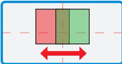
Turning the Split control anti-clockwise will separate the two images along the horizontal axis. Only small adjustments will be required when using the horizontal image separation adjustment.
