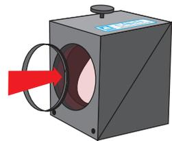
Replace the locking ring and rotate it clockwise to secure.
