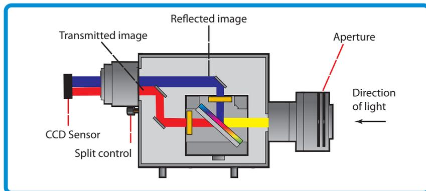
The design is loosely based on technology described by Kinosita et al. (J.Cell Biol. [1991] 115, 67-73), but includes several proprietary features, most notably:
