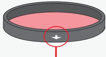
The arrow should be orientated into the filter cube and towards the light path.
