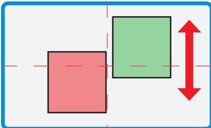
Should the left and right images be at different vertical heights then adjust the images using the V1 and V2 adjuster. Turning V1 will alter the position of the shorter wavelength image, and V2 will alter the position of the longer wavelength image.
