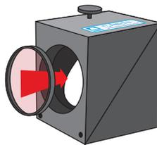
Carefully place the filter inside the recess.
