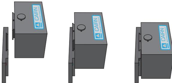
Mount the filter cube onto the bracket on the interior of the Optosplit II.
