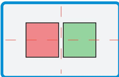
When the spectrally resolved images are side by side on the camera chip you are ready to record. When carrying out experiments the aperture should be set to mask the region of interest tightly so that the two images are located as closely as possible on the camera chip.
