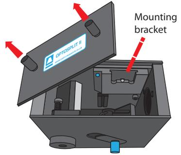
Remove the access panel using the two handles.
