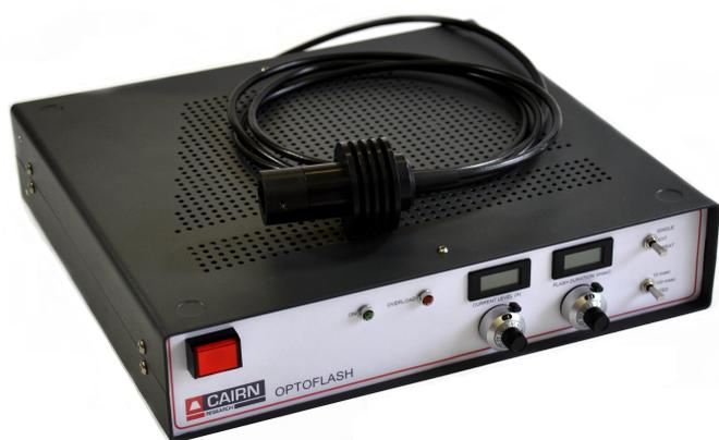
We have decided to make the Optoflash a single-channel design, rather than being able to drive two LEDs independently as the OptoLED does. However, the price difference does take this into account, and multiple units can easily be stacked if required. Also note (and see further below) that a single Optoflash may be capable of driving multiple optical fibres at the same time.
