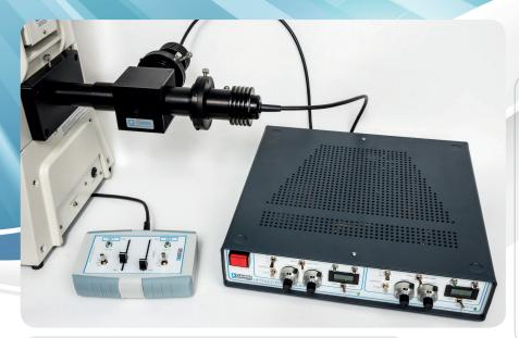
High intensity LEDs are now available across the visible spectrum extending into both the ultraviolet and infrared. Their fast switching, longlife, high stability, variable intensity and lower power consumption make them ideal for both fluorescence and transmitted light microscopy. The Cairn OptoLED system has been designed to best exploit this new technology whilst maintaining compatibility with arc lamp and laser illumination sources.
